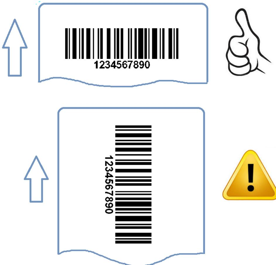
For barcodes with bars not parallel to the printing direction, increase the magnification by at least 1 point and reduce the printing speed.
